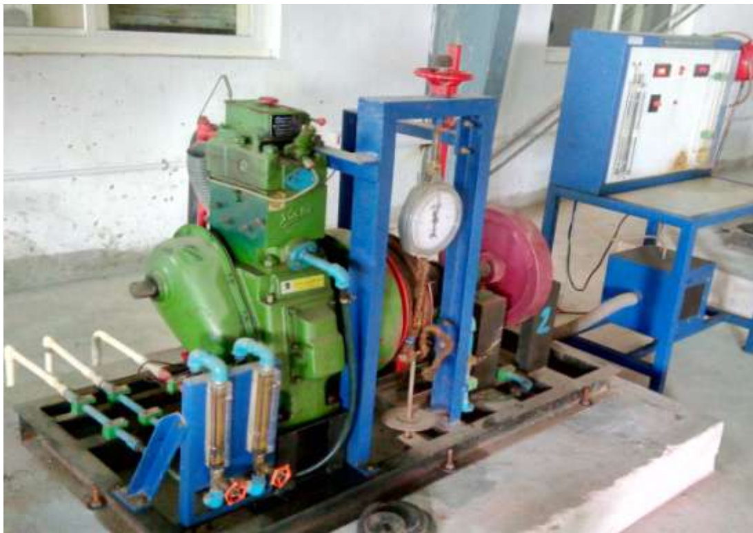
Fig.6.Four stroke single cylinder direct injection diesel engine
