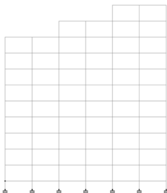
FIG Elevation & 3D View of RCC G+10 building with setback on plain ground
