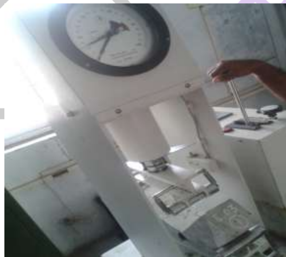
Figure 3- Flexure Test in Progress
