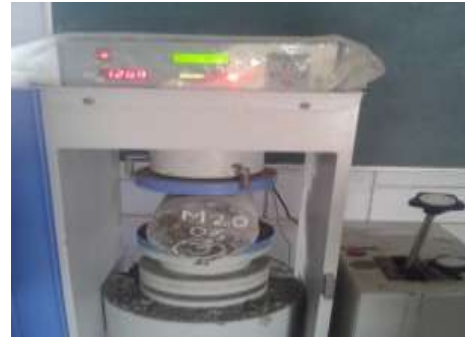
Figure 2- Split Tensile Test in Progress
