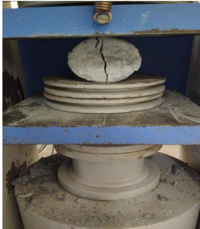
Fig. 2 “Testing of Split tensile strength test specimen”
