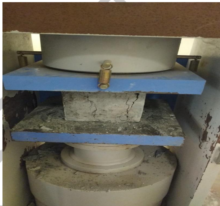
Fig. 1 “Testing of compressive strength test specimen”
