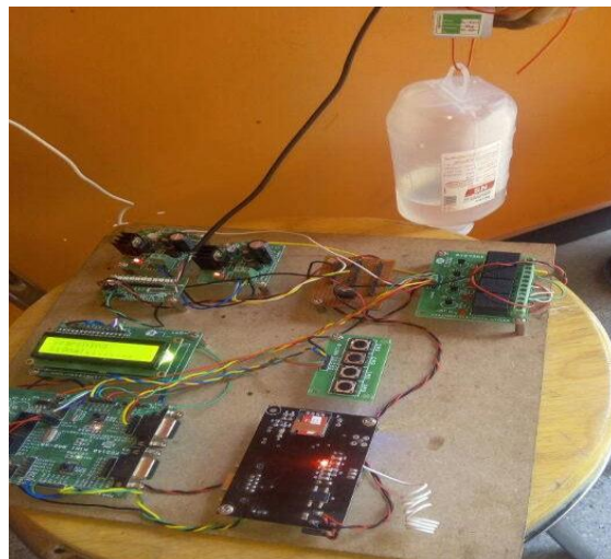
Fig 3. Model of Saline level Monitoring and Control System
