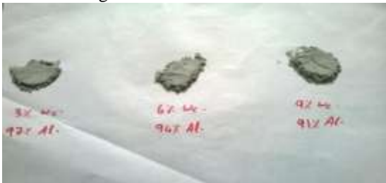
Fig7: different compositions of Al-Wc
