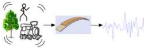
Figure 1: Vibrational energy is apparent everywhere. One method to harvest the Vibrational energy is to mount a piezoelectric material in the vibrating environment. During motion, the piezoelectric material will generate an AC voltage.
