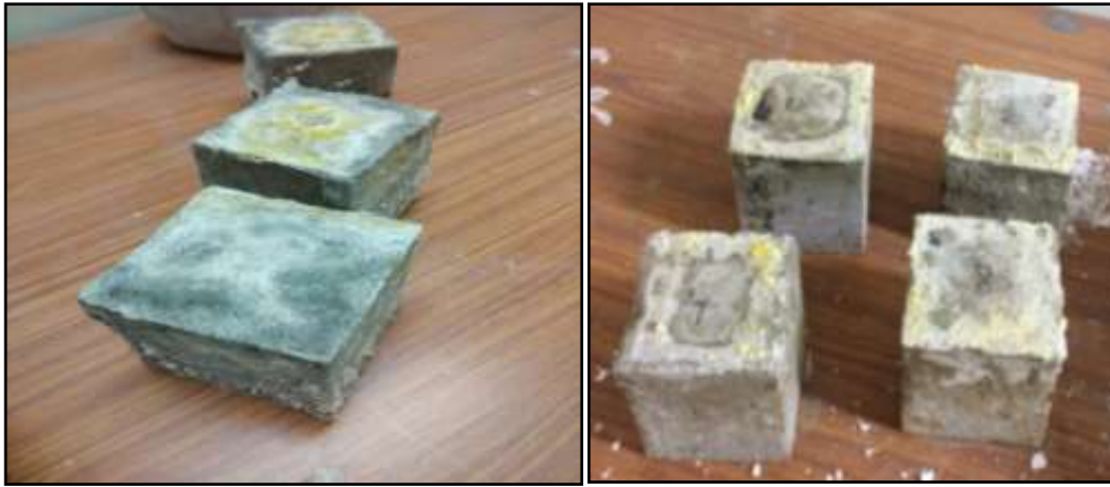
Figure 23: Visual appearance of GPC-N specimens
