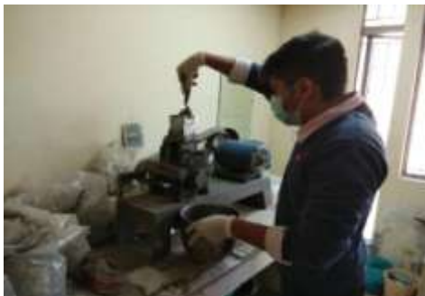
Figure 1: Casting on vibrater
