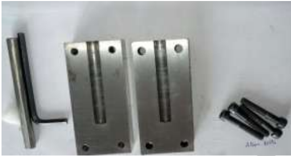
Fig. 2.HCHC-D3 steel Die and Punch
