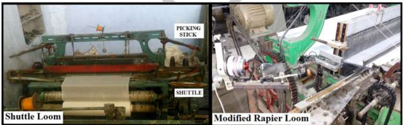
Figure 1: Weaving by Shuttle Loom and Modified Rapier Loom
