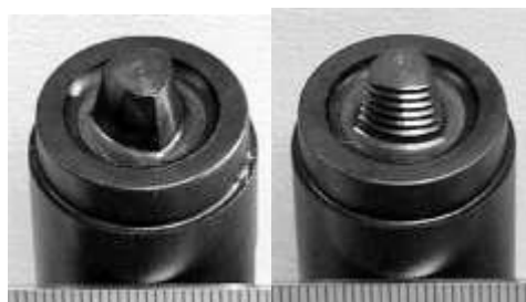
“Fig.3” Trivex series design of FSW tool.
