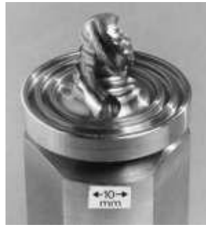
“Fig.4” Triflute series design FSW tool.
