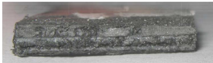
“Fig.8” Tunnel defect in stir zone.
