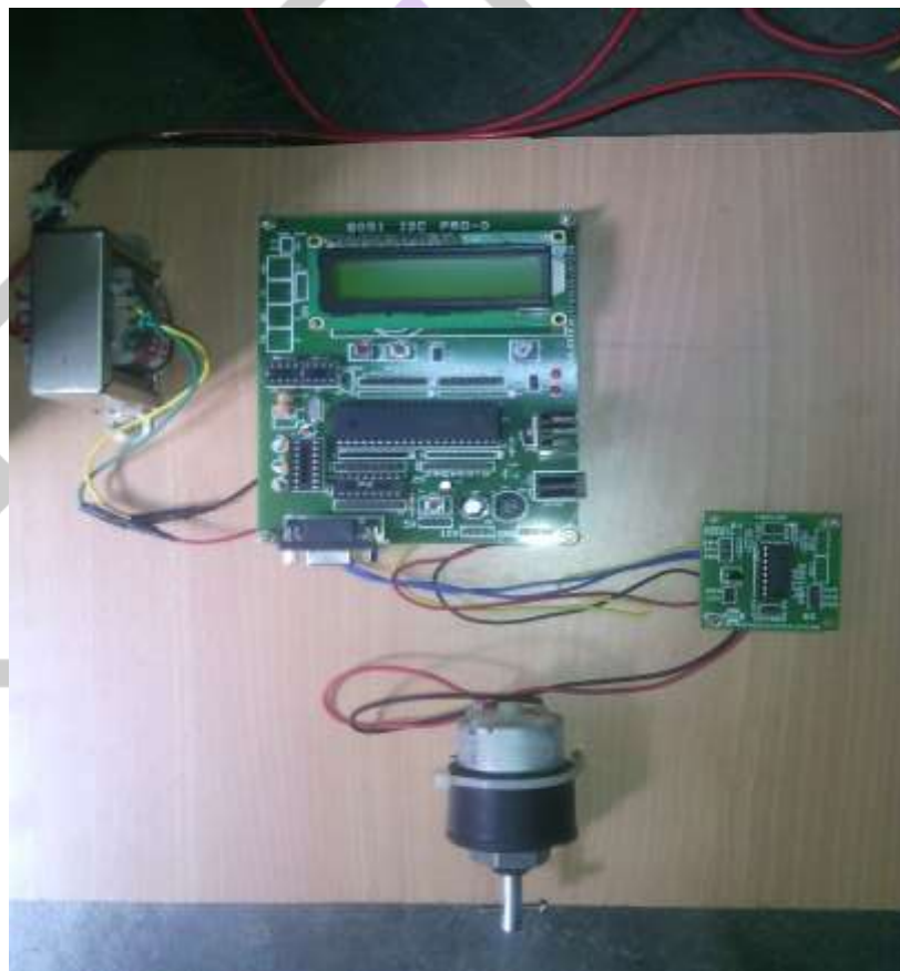
Fig. 4.5: Dc Motor Controlled by Microcontroller
