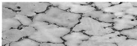
Fig- 12 Phosphors % higher at grain boundry as Phophite. Not accepted structure (> 0.05% P)
