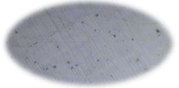
Fig.9 microstructure shows Austenitic grain and Mn carbide
