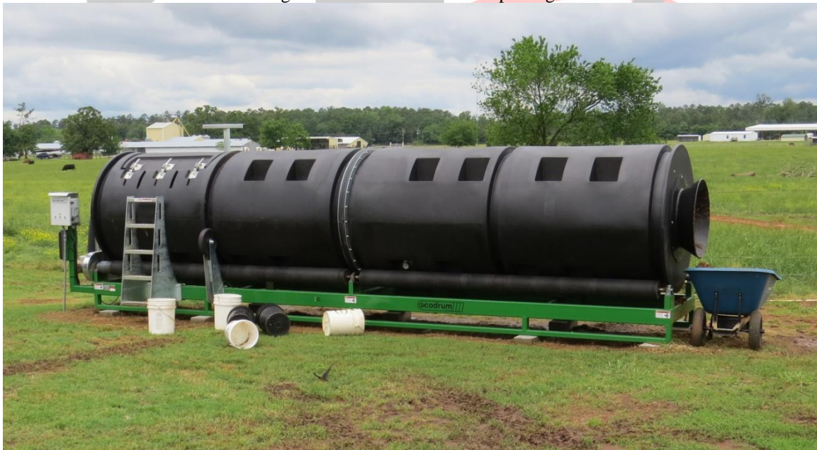
Figure 3 Enclosed Vessel Composting
