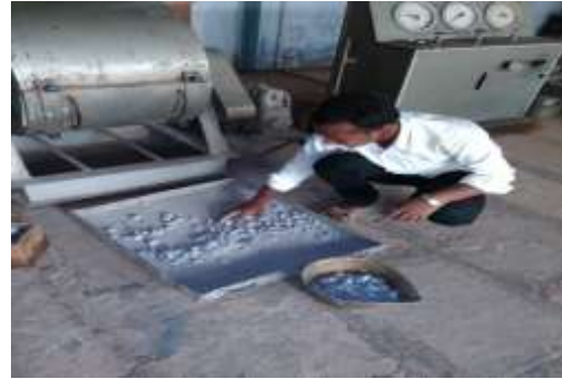
Fig. 5 Aggregates obtained after milling
