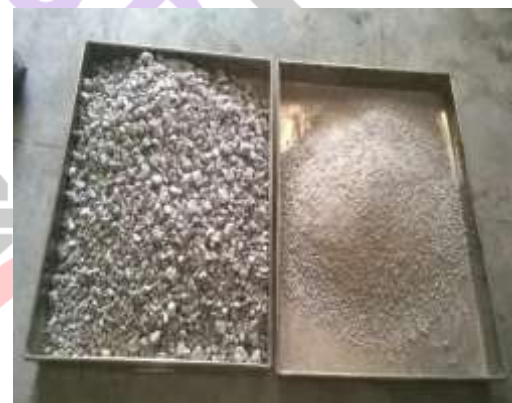
Fig. 7 Aggregates after heating and scrubbing
