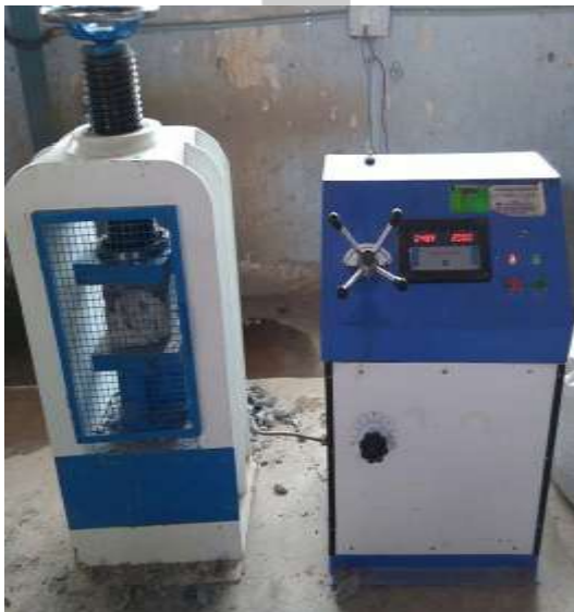
Fig. 10 Testing cube specimen
