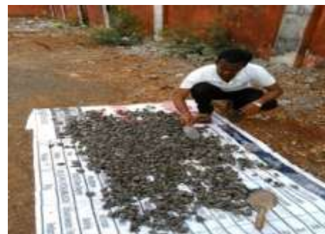
Fig. 9 Drying cement coated aggregates
