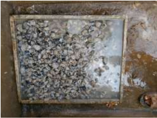
Fig. 4 Washing aggregates after soaking
