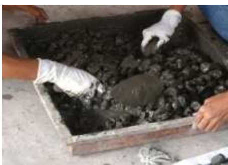
Fig. 8 coating with cement slurry
