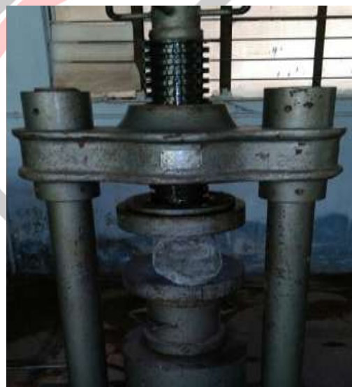
Fig. 11 Cylinder specimen loading along the length
