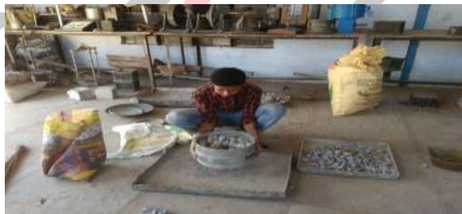
Fig. 3 Sieving broken aggregate through standard sieves
