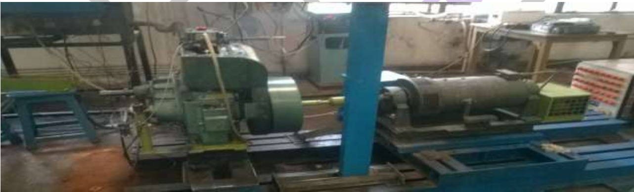
Figure 5.2: Kirlosker four stroke Single cylinder vertical air cooled engine
