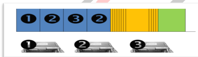
FIG. 5.3- ILLUSTRATION OF A STATIC SEGMENT WITH 3 ECUS TRANSMITTING DATA TO 4 RESERVED SLOTS.
