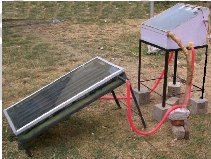
Fig 1: Experimental setup of solar still (23°) with collector
