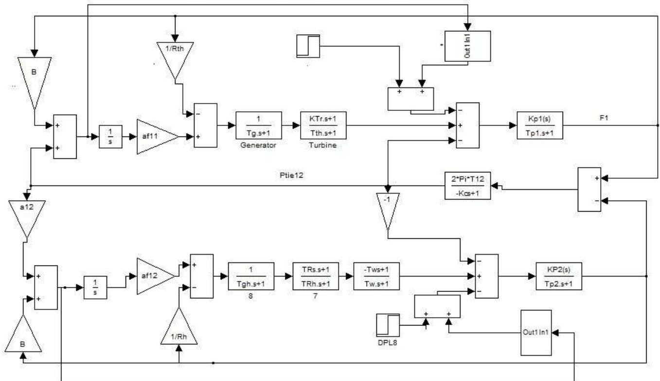
fig 3 interconnected power system model with SMES
