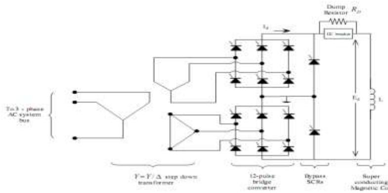
Fig. 1. SMES circuit diagram
