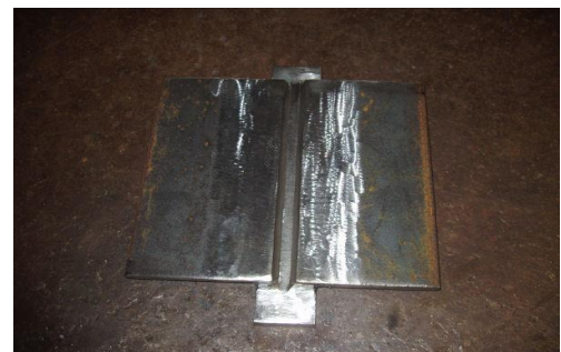
Fig 2 : Weld between Stainless steel and mild steel
