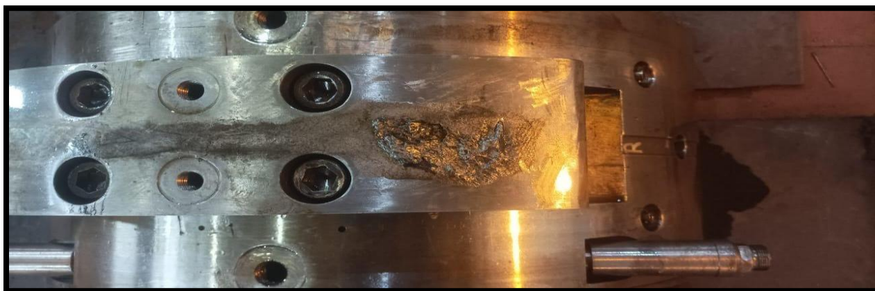
Figure 3: Electrical discharge markings at bearing torus support.
