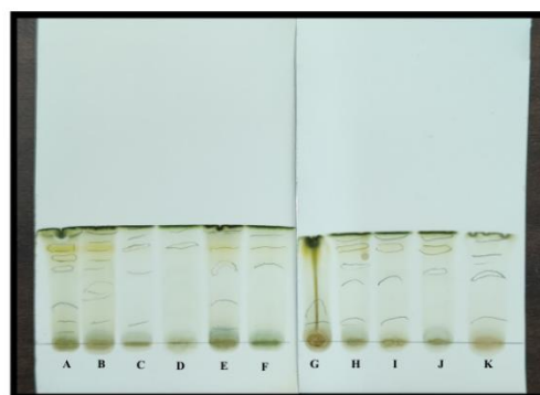
2.TLC plate under visible/white light
