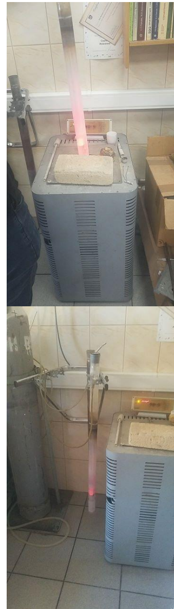
Figure 18 – Annealing process of Cu-Ni ingots at 900°C
