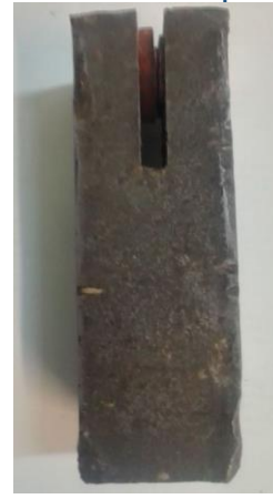
Figure 23b – Cu-Ni and Cu-Sn-Ni diffusion couple Assembly Set-up
