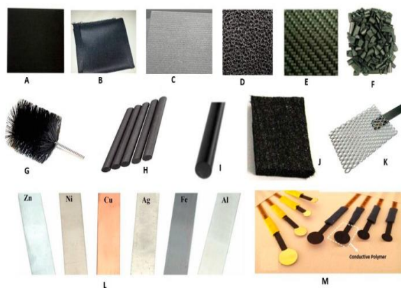
Figure 5 – Other commonly used electrodes for anode and cathode in MFCs [23]
