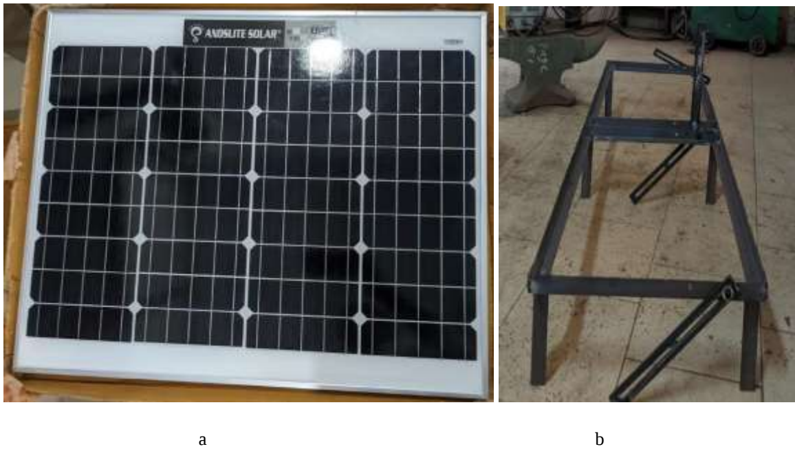
Figure 1: (a) 50W 12V photovoltaic panel (b) Tiltable stand for keeping the photovoltaic panel.
