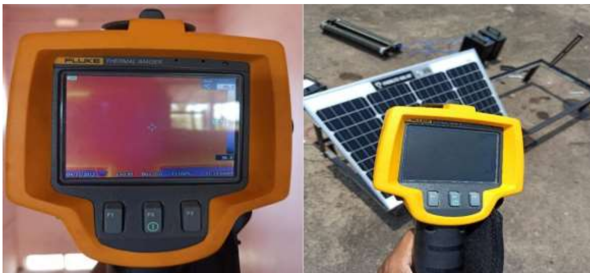
Figure 2: Thermal camera used for measuring the temperature developed on the PV panel
