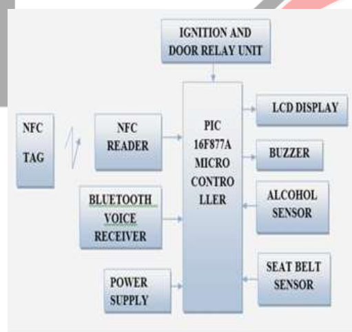
Figure 4.1: Block diagram of Proposed System
