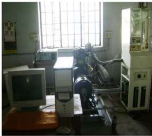
Fig.III.3. Experimental setup of computerized CI Engine
