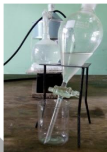
Figure (2) The extracted oil by using separating funnel
