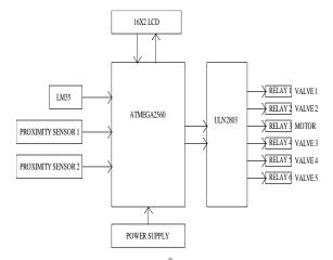
ATMEGA 2560 microcontroller is used to operate the machine. LM35, proximity sensor 1. Proximity sensor 2 are connecting with ATMEGA2560. 5V power supply is given to the ATMEGA 2560. Relays are used to operate the valves and motor.
