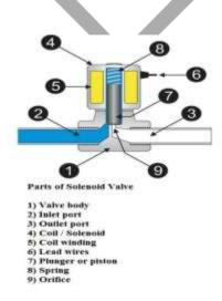
A solenoid valve is an electromechanically operated valve. The valve is controlled by an electric current through a solenoid. Here, in this case a two-port valve is used in which the flow is switched on or off. It basically works as an actuator for the system.
