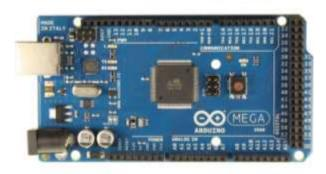
The Arduino Mega 2560 is a microcontroller board based on the ATmega2560. It has 54 digital input/output pins (of which 15 can be used as PWM outputs), 16 analog inputs, 4 UARTs (hardware serial ports), a 16 MHz crystal oscillator, a USB connection, a power jack, an ICSP header, and a reset button. It contains everything needed to support the microcontroller; simply connect it to a computer with a USB cable or power it with a AC-to-DC adapter or battery to get started.
