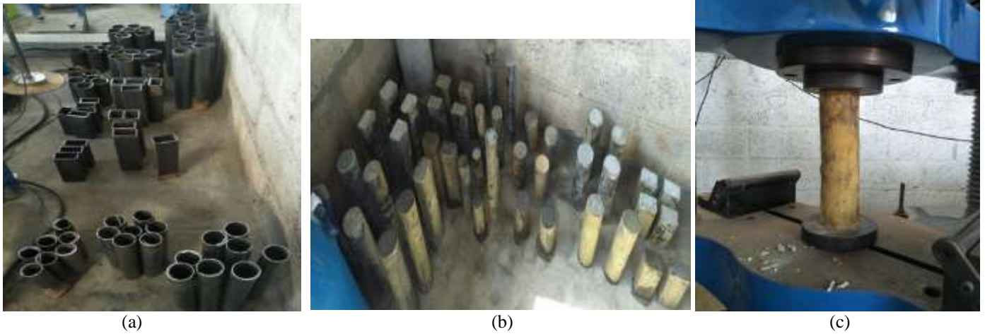
(a) Empty columns before casting (b) Filled steel columns after curing (c) Steel column testing in UTM
