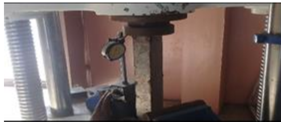
Figure 4.Buckling Behavior of specimen due to load
