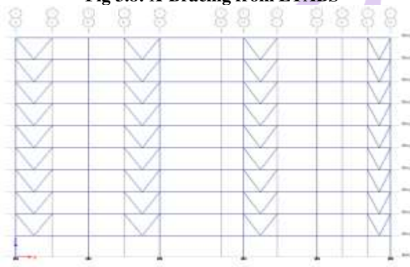
Fig 3.9: V Bracing from ETABS
