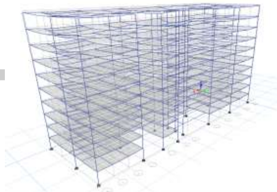
Fig 3.17: 3D-Deformed shape from ETABS
