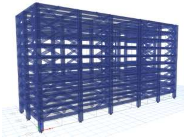
Fig 3.11: 3D view X Bracing from ETABS
