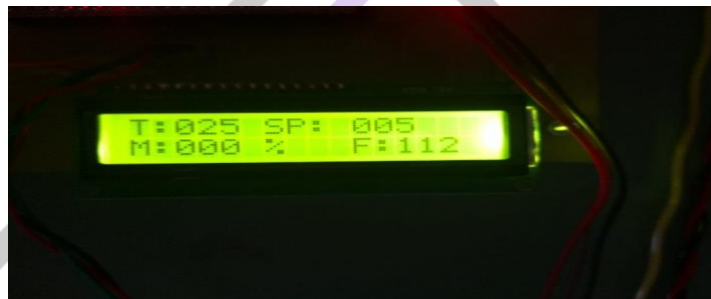
Fig 5. LCD display shows values of temperature, Moisture, flow and set point
