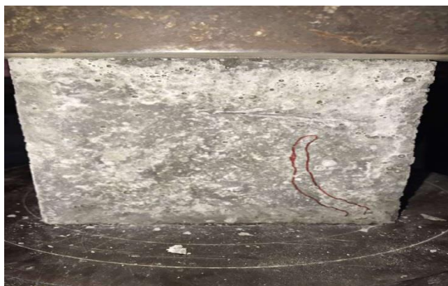
Image No.3 Concrete block under compression
