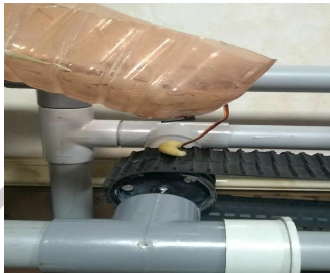
Fig. 4 The Cashew kernel being Dropped on the Conveyor Belt
