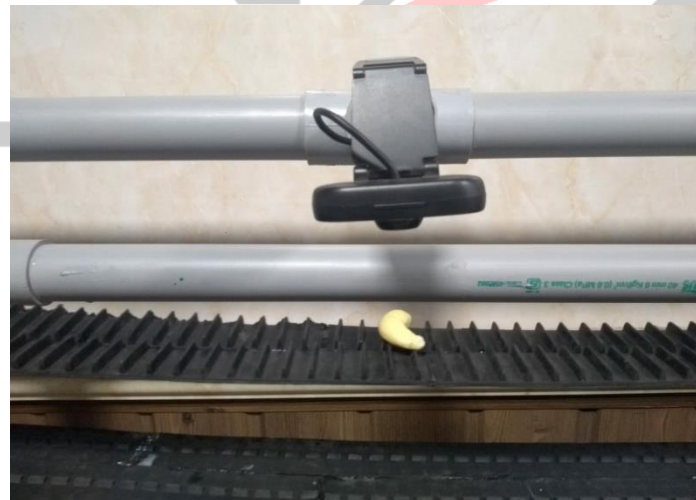
Fig. 5 Camera Capturing the Image of Cashew Kernel
