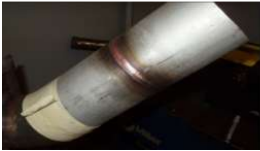
Fig 3.1 : Normal TIG welding
