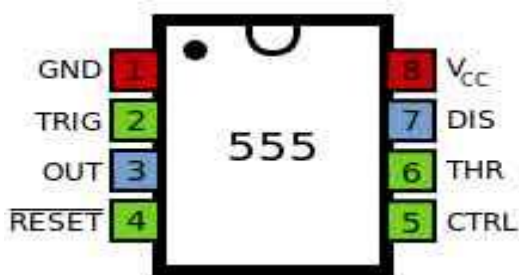
Fig 1.6: IC 555 timer pin diagram
