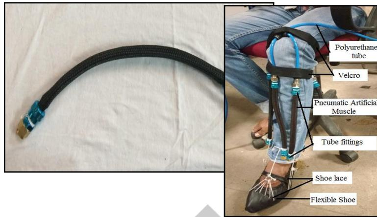
Fig. 1. Pneumatic Artificial Muscle. Fig. 2. Experimental model.
