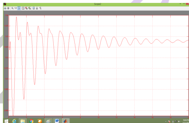
Fig. 6. Voltage at bus 2 without SSSC
