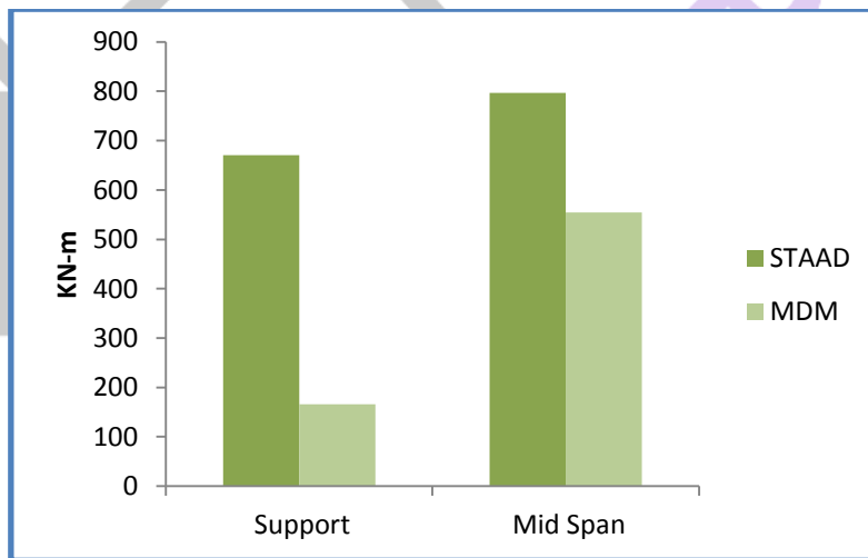
Figure 4: Comparison of STAAD and MDM results for Deck Slab
