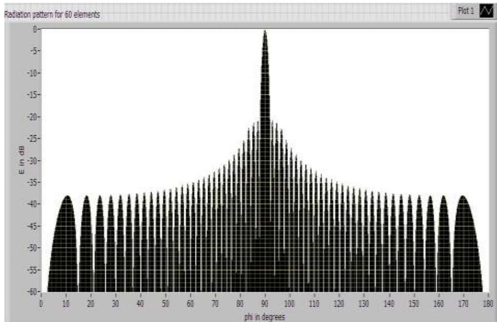
Figure 6: Radiation Pattern with  $\bar{n} = 4$  for 60 elements in LABVIEW
