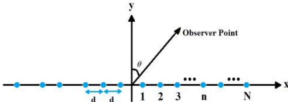
Figure 1: Geometry for symmetric structure of linear array
