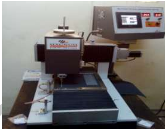
Figure 1. Schematic diagram of multi-pass two body abrasion machine tester rig.
